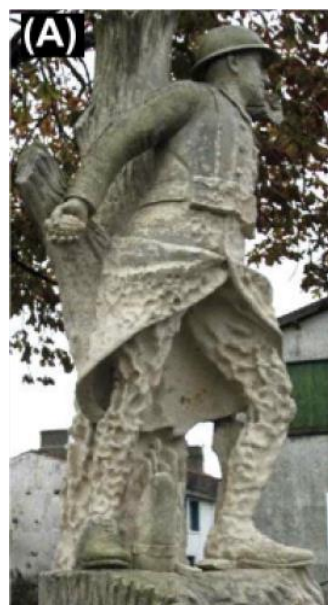
Left: erosion damage on a statue from salt crystallization. Right: nucleation and growth of various forms of NaCl crystals nucleated in an elongated droplet at 160% of the equilibrium solubility
