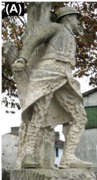
Left: erosion damage on a statue from salt crystallization. Right: nucleation and growth of various forms of NaCl crystals nucleated in an elongated droplet at a concentration 60% higher than of equilibrium solubility.
