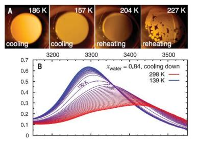
Optical observation of the solutions and infrared spectra recorded during cooling [5].
