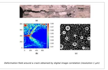
[Richeton] that plasticity is intermittent because of plastic avalanches. It is therefore possible that acoustic emission (AE) signals, that were attributed to rupture events [Lii], stem from plastic avalanches. As a consequence, a fine characterisation of the plasticity occurring during crack propagation is required.
