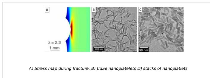
A) Stress map during fracture. B) CdSe nanoplatelets D) stacks of nanoplatelets
