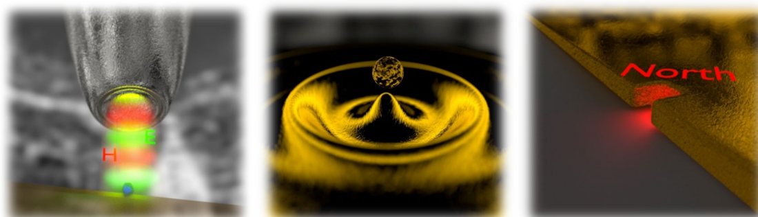
Figure 1: (left) Standing wave generation with a SNOM set-up, allowing the controlled electric or magnetic excitation and emission. (center) Coupling between the matter and the magnetic part of the localized plasmon. (right) A newly designed antenna which behaves like a magnetic monopole. Credits: M. Mivelle.
