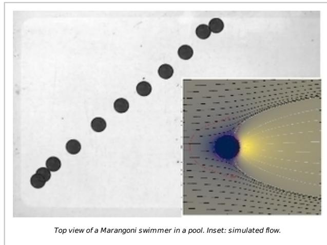
Top view of a Marangoni swimmer in a pool. Inset: simulated flow.
