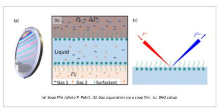
contrary to solid membranes. These properties are crucial to new **energy-efficient chemical separation processes**, currently corresponding to 10-15% of worldwide energy consumption. Separation devices have to be selective to one of the gas species, and this can be achieved in soap films thanks to the specific **adsorption of gas species on the surfactant layer**.
