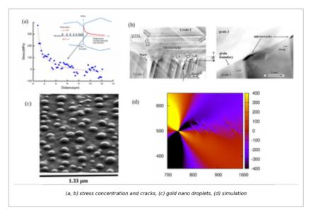
might be activated at the tip of slip bands when those are blocked by obstacles, such as grain boundaries (Fig. 1) and lead to the formation of crack embryos [10-12]. Even if the existence of stress concentrators is well known, in situ observations are scarce [12,13].
