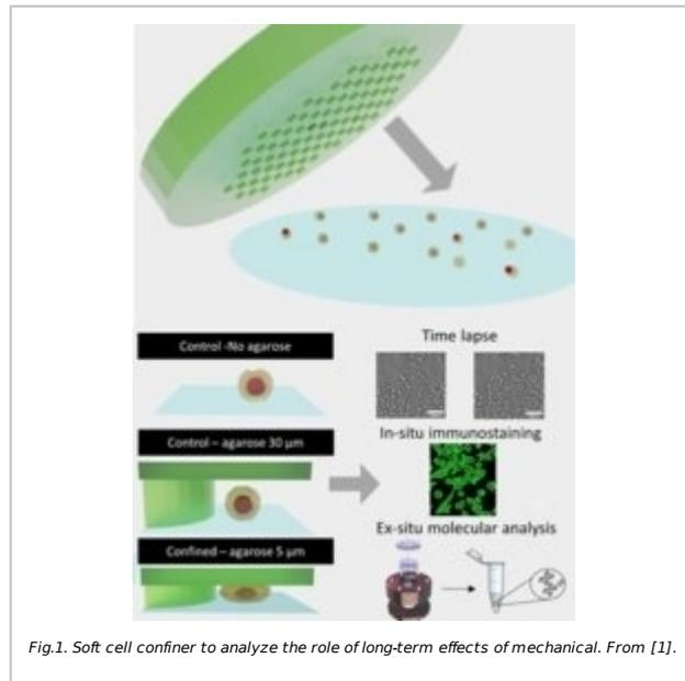
Fig.1. Soft cell confiner to analyze the role of long-term effects of mechanical. From [1].
